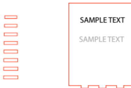
Caption: Test Illustrator file for laser cutting. (Left) varying peg hole sizes. (Right) varying rastering levels of text.
